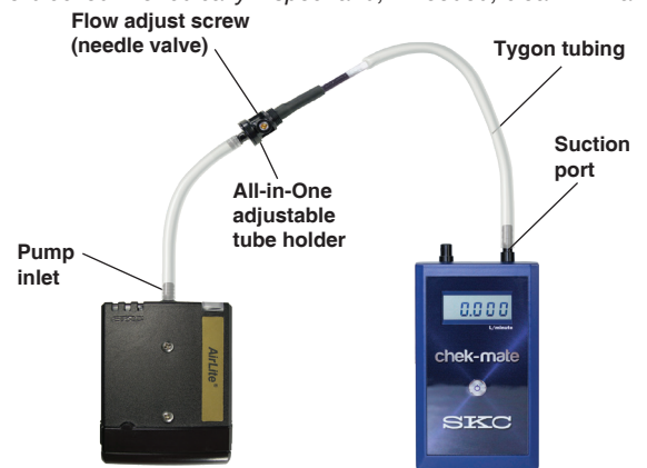
Calibration train with All-in-One connected to pump
