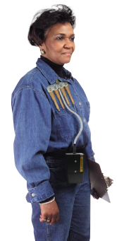
Clip tube holder to worker and pump to belt.
