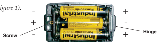
Polarity of batteries
